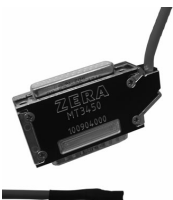
MT3450, Temperature sensor Sensor for measuring of the ambient temperature on site. The measured temperature value is displayed and saved in the MT device. Temperature range: -20° C ... +60° C (± 1° C) Resolution: 0,1° C Cable length: 3 m
